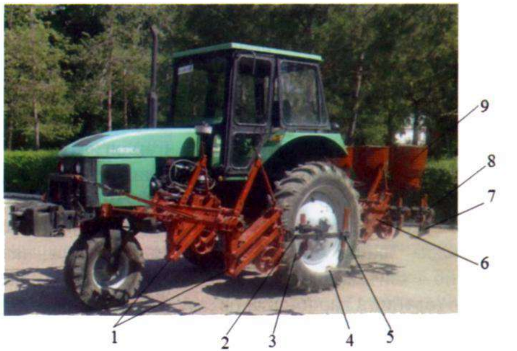
1-section attenuator; 2-gryadyl; 3- softening working Body; 4-tractor leading wheel; 5-lock; 6-parallelgramm mechanism; 7-socket; 8-handle with sterjen; 9-fertilising apparatus;
